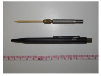
Figure 2. Comparison of dimensions between the mandrel-toothpick assembly and a common ballpoint pen.
