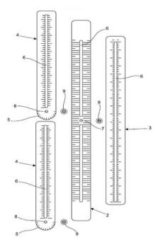
**Figure 2.** Exploded diagram of the abdominoplasty marking instrument.
