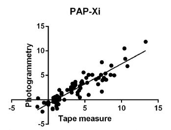
Figure 6. Very strong correlation between photogrammetry and tape measure.
